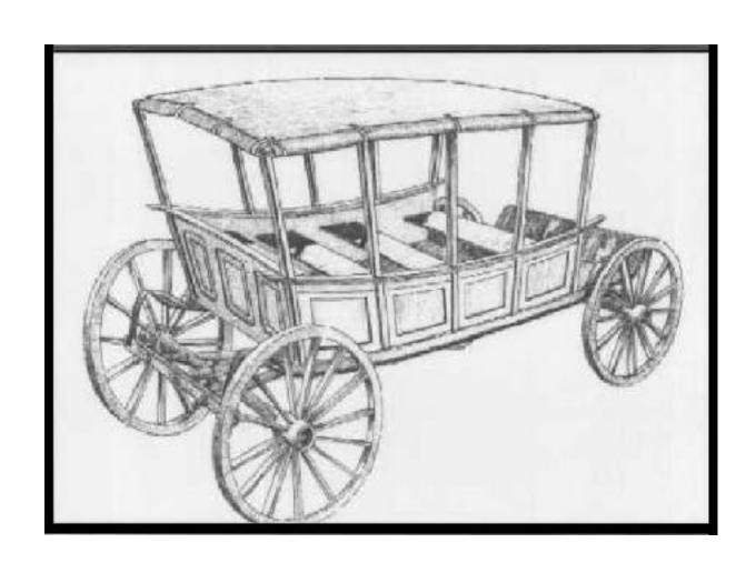
**Stage coaches**, replaced "waggons" in the late 1700s. They were much more comfortable not only because they had doors and windows but they had suspension as well. Carriages were attached to the chassis by leather straps so that every rut and rock was a bit less bone-rattling. This small stage coach ran in South Jersey and is now at the Batsto Village museum.
